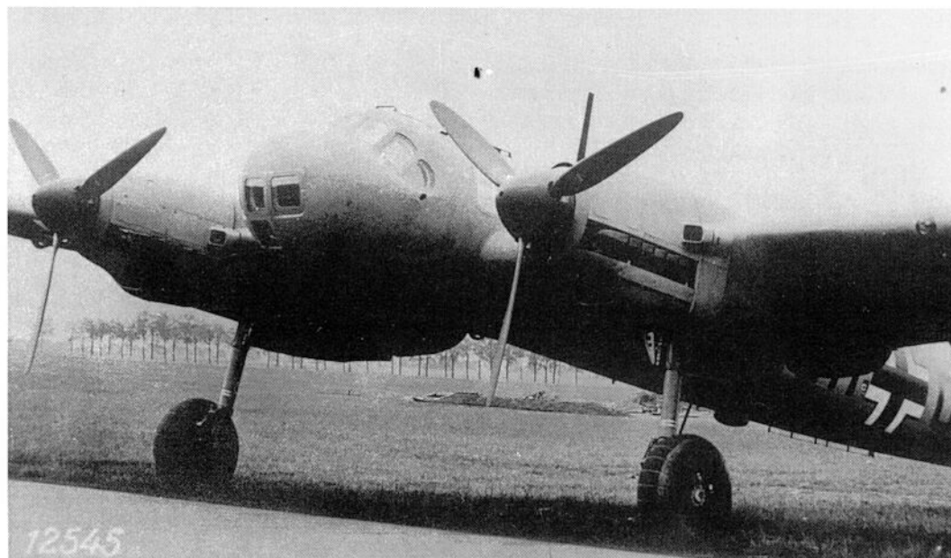
Left: The majority of Hs 130 A-0s built were powered by two DB 601 R-0 engines fitted with the GM-1 nitrous oxide injection system. Testing began in August 1940.
