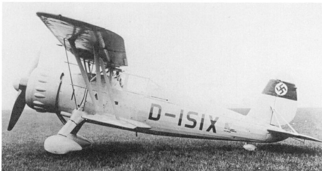
Left: The Ar 68H, seen here in spring 1937, differed from the Ar 68F in having a BMW 132 Da radial.
