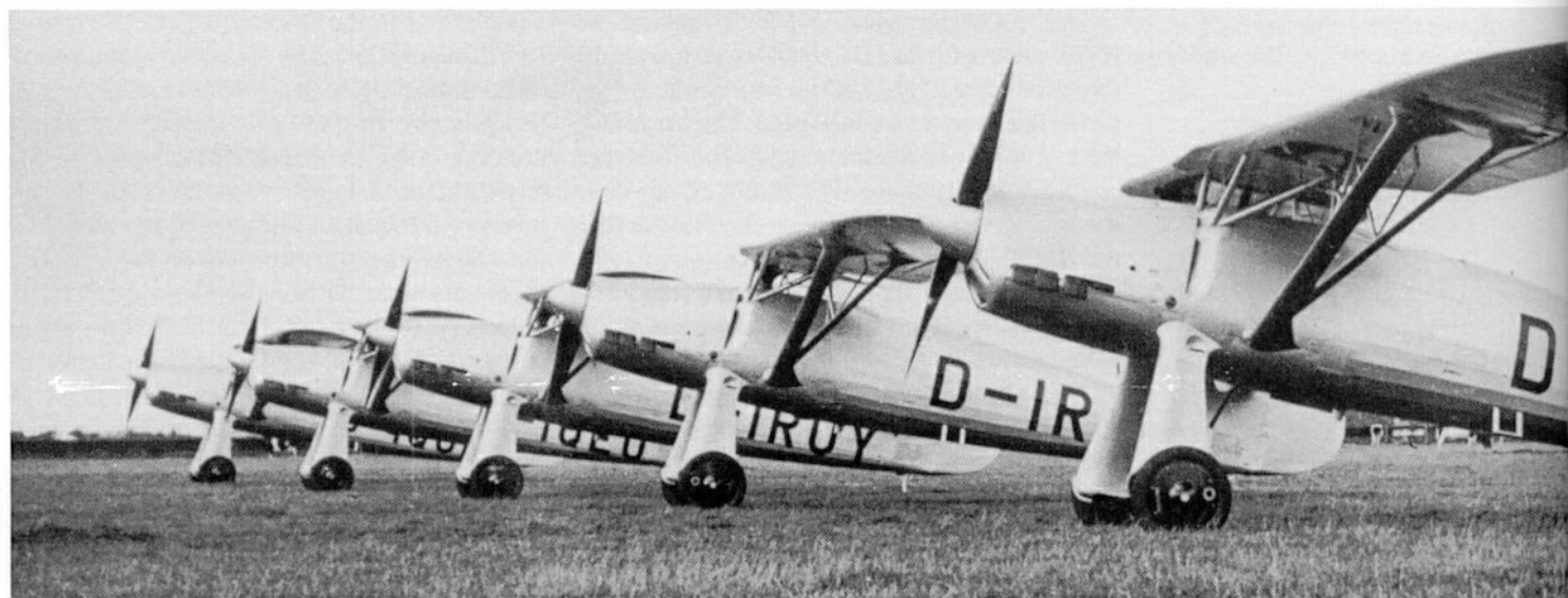
Below: Focke-Wulf developed the Fw 56 as a trainer and escort fighter; about 1,000 of these machines were built.
