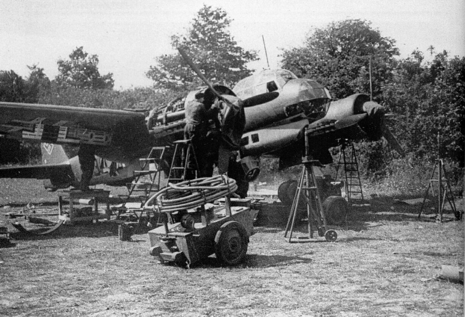
Above: Maintenance work on a Jumo 211 in-line engine of a Ju 88 A-5 of KG 54. Note the extended dive-brakes.
