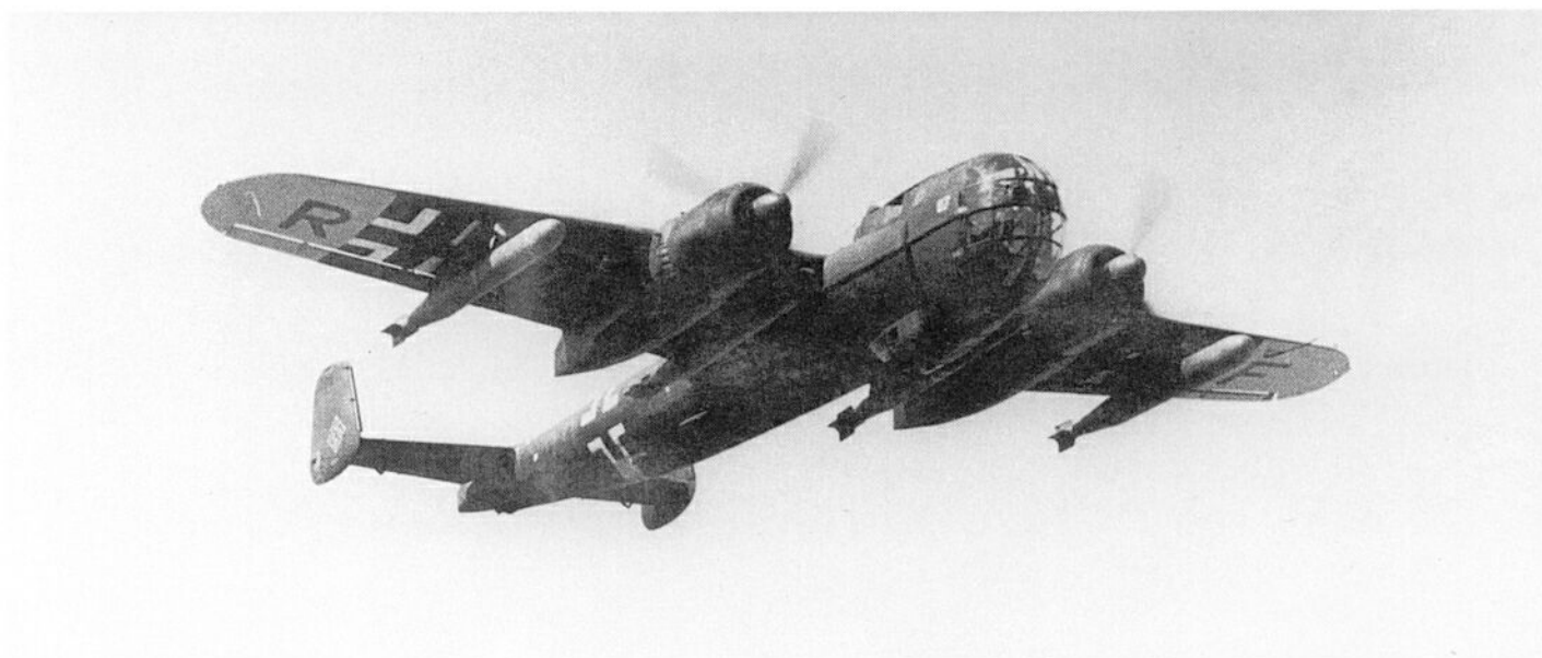
Above: The Do 217 K-07 (Works No.4407, RD+JF) was used from January 1943 as a torpedo bomber, carrying up to four LTF 5s.
