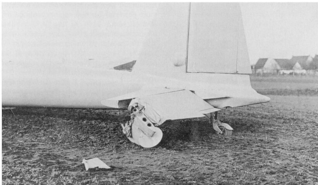
Left: Crash landing of the Fw 187 V1 due to landing gear failure.
