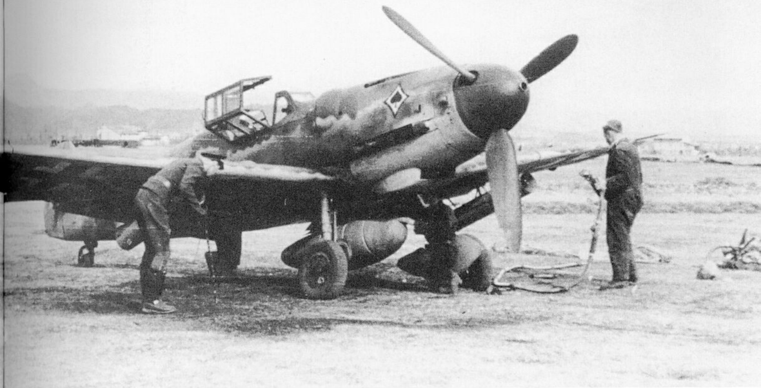
Above: A Bf 109 G-6 of JG 53 equipped with a 300-litre drop-tank and two WGr 21 rocket-launchers.
