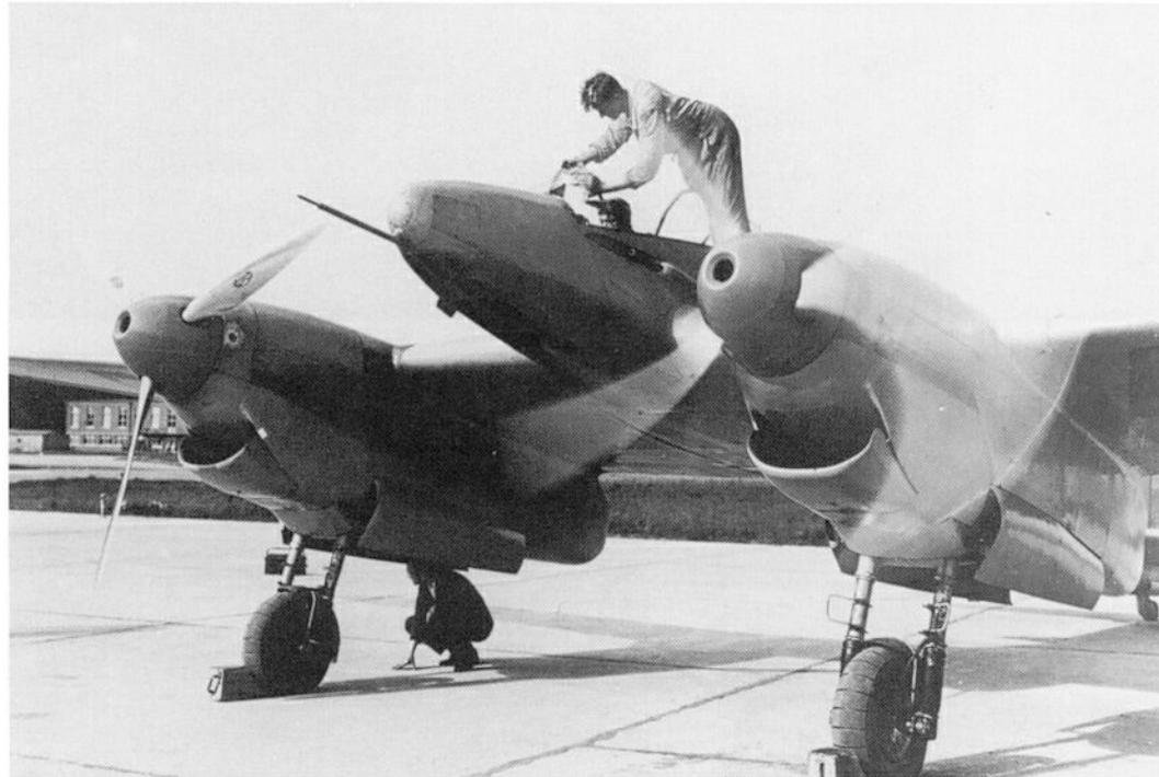
Left: A twin-engined heavy-fighter of superior performance was the Focke-Wulf Fw 187 V1 (Works no 949), which was 35km/h faster than the Bf 109.
