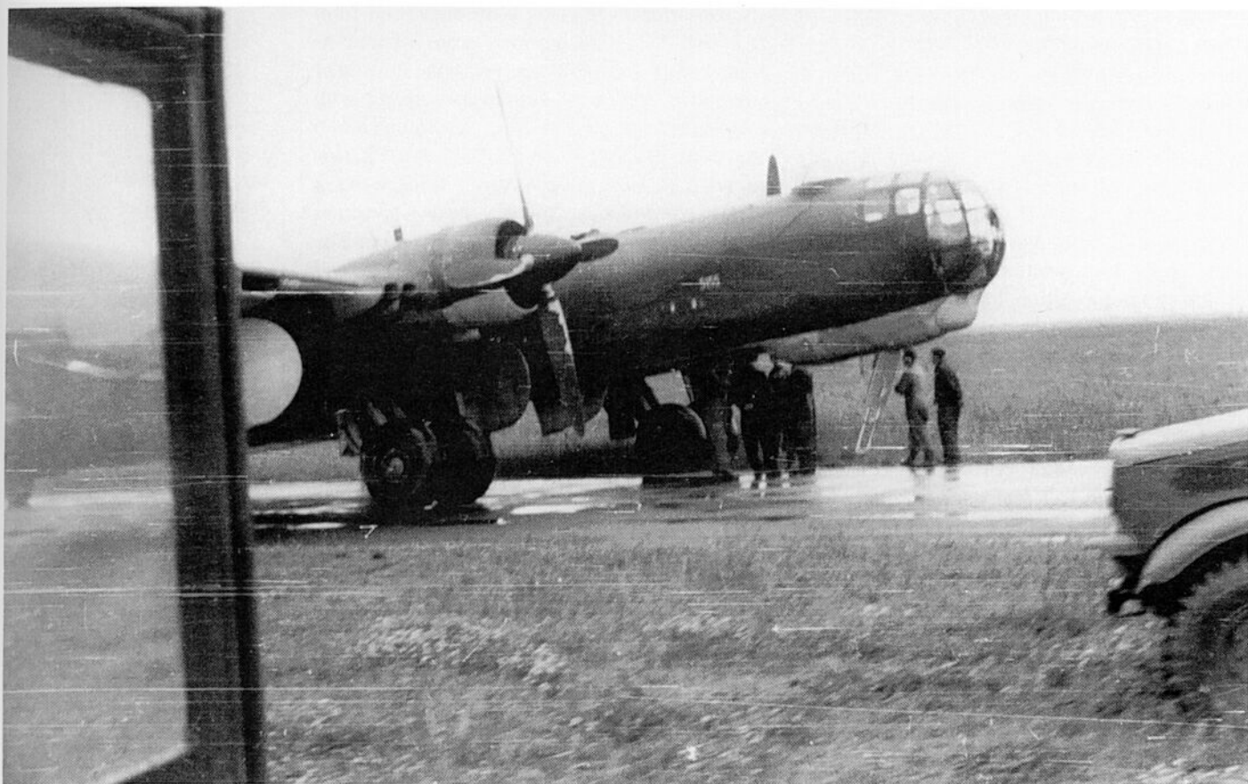
Above: A remote-controlled nose gun position was tested on this He 177 A-1 (Works No.15155) at Rechlin experimental establishment.
