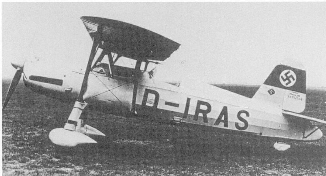
Left: The Ar 76 was developed as a 'home defence fighter'. This photograph shows the Ar 76 V2 (D-IRAS), armed with two MG 17s.
