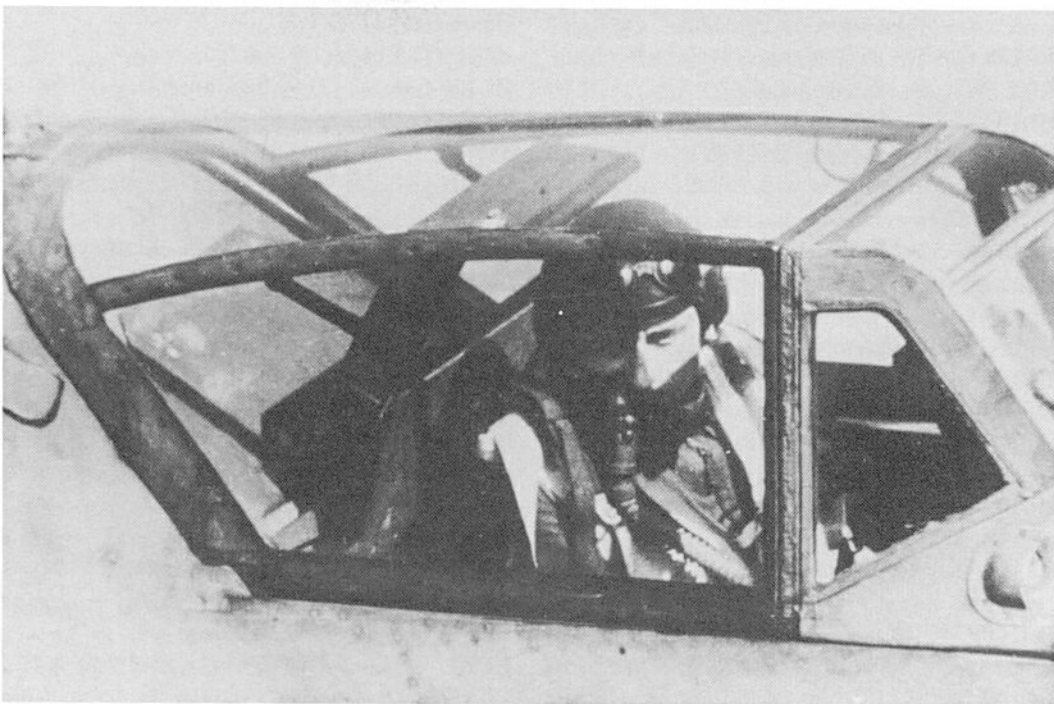
Left: A Bf 109 G-14AS with the so-called 'Erla Canopy', sometimes wrongly called the 'Galland Canopy', and armoured rear protection for the pilot.
