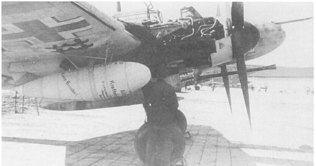
Right: A Bf 110 G-2/R4 with two MG 151/20s in place of the previous nose armament, as well as a 37mm cannon mounted beneath the fuselage, seen at Munich-Riem in June 1944).
