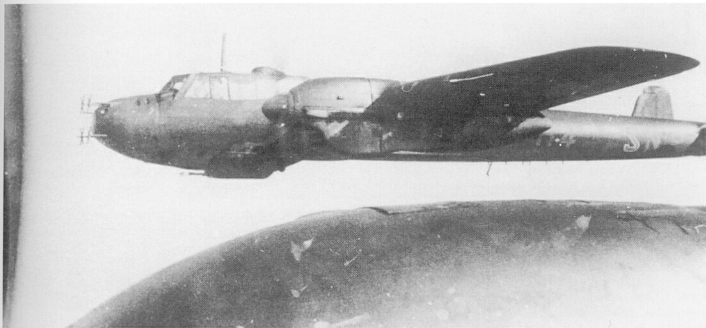
Above: Two Do 215 B-5 night fighters of 5./NJG 5 during a formation flight. The aircraft in the background has an two additional 20mm cannon fitted below the forward fuselage.
