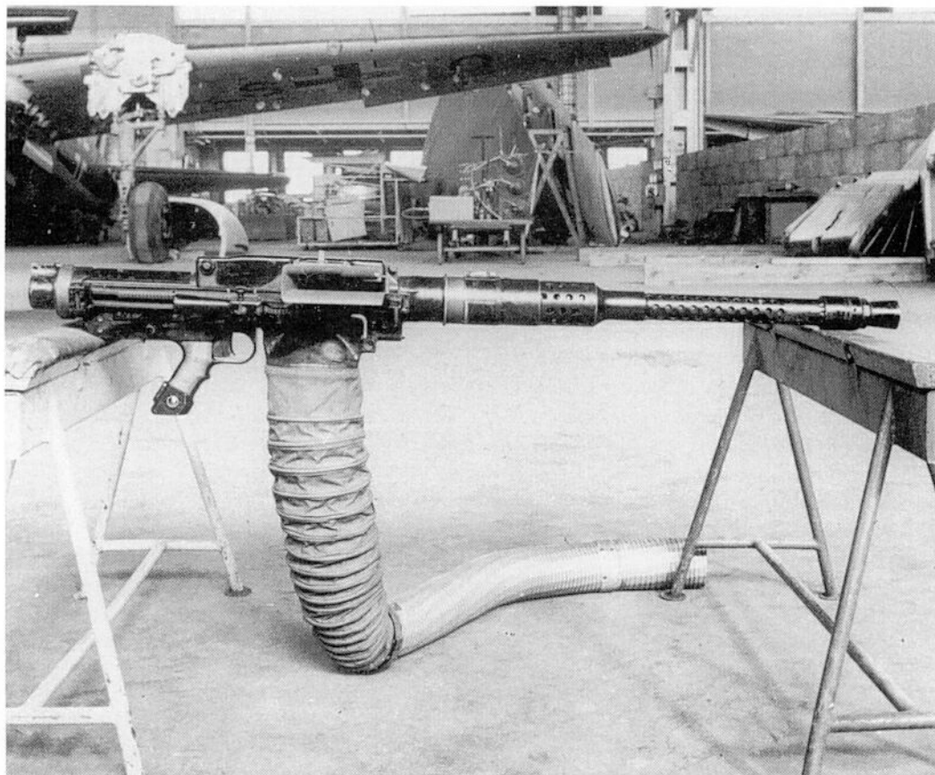
Left: Side view of an MG 131 I, which was intended to be used, for example, in the Ju 188 E-1 or the planned G-2.
