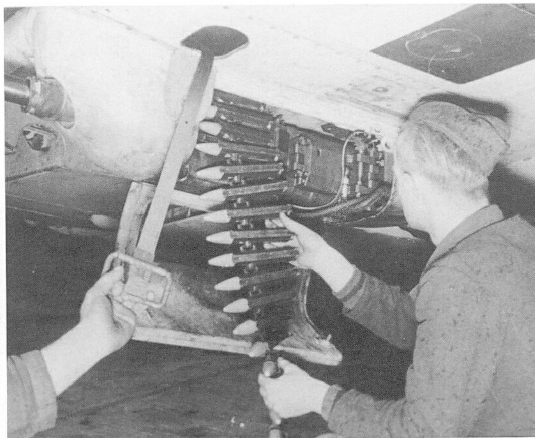
Left and above left: In place of the two MG 151/20s, two MK 108s could be used in underwing gondolas. This photograph shows the prototype for the Bf 109 G-6/U4 series.
