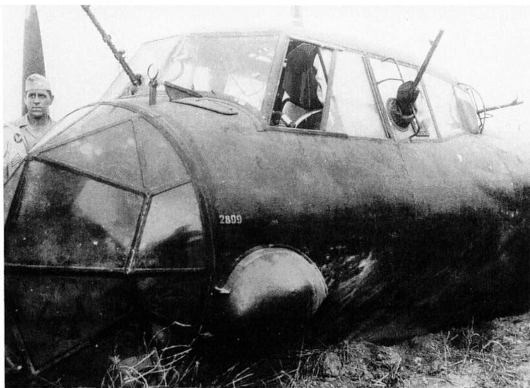
Above: The heavily-armed Do 17 Z-5 was a conversion of the Z-2, and carried inflatable flotation bags for emergency ditchings.
