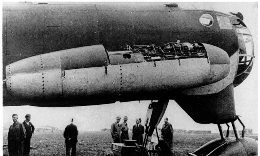
Right: The Ju 287 V 1 was powered by four Jumo 004 B-1 turbojets, with three rockets for assisted take-offs.
