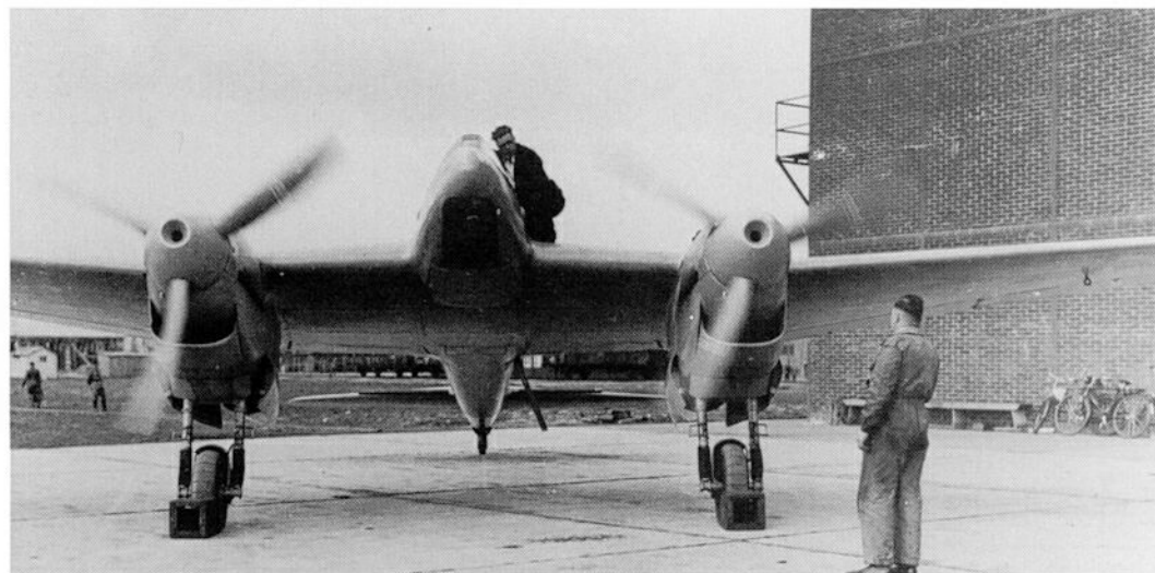
Left: The Fw 187 V2 was armed initially with two MG 17s. During the course of testing, engine power was improved by replacing the two Jumo 210 Da engines with two Jumo 210 Gs.
