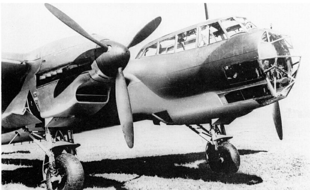
Left: The Do 215 B-2 was a four-seat medium bomber with six MG 15s as defensive armament.
