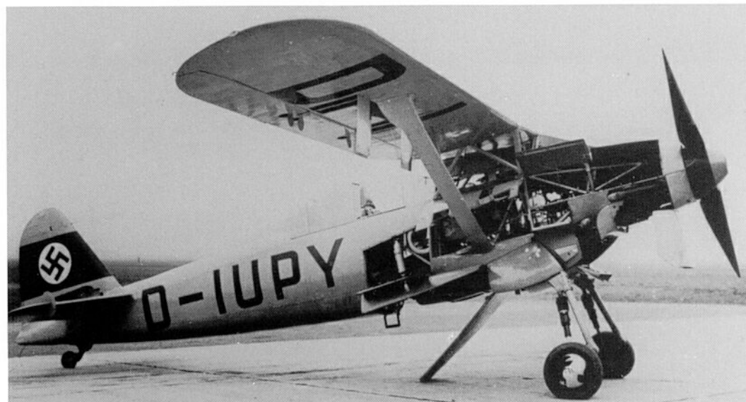
Left: The high-wing Fw 159 fighter, here seen in its V1 version (D-IUPY), was intended to be fitted throughout with the Jumo 210 B engine.
