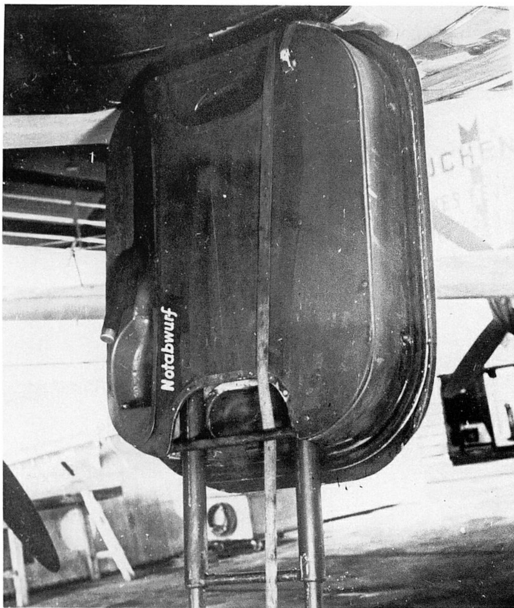
Left: The cabin hatch of the Ju 388 J-1, K-1, and L-1.
