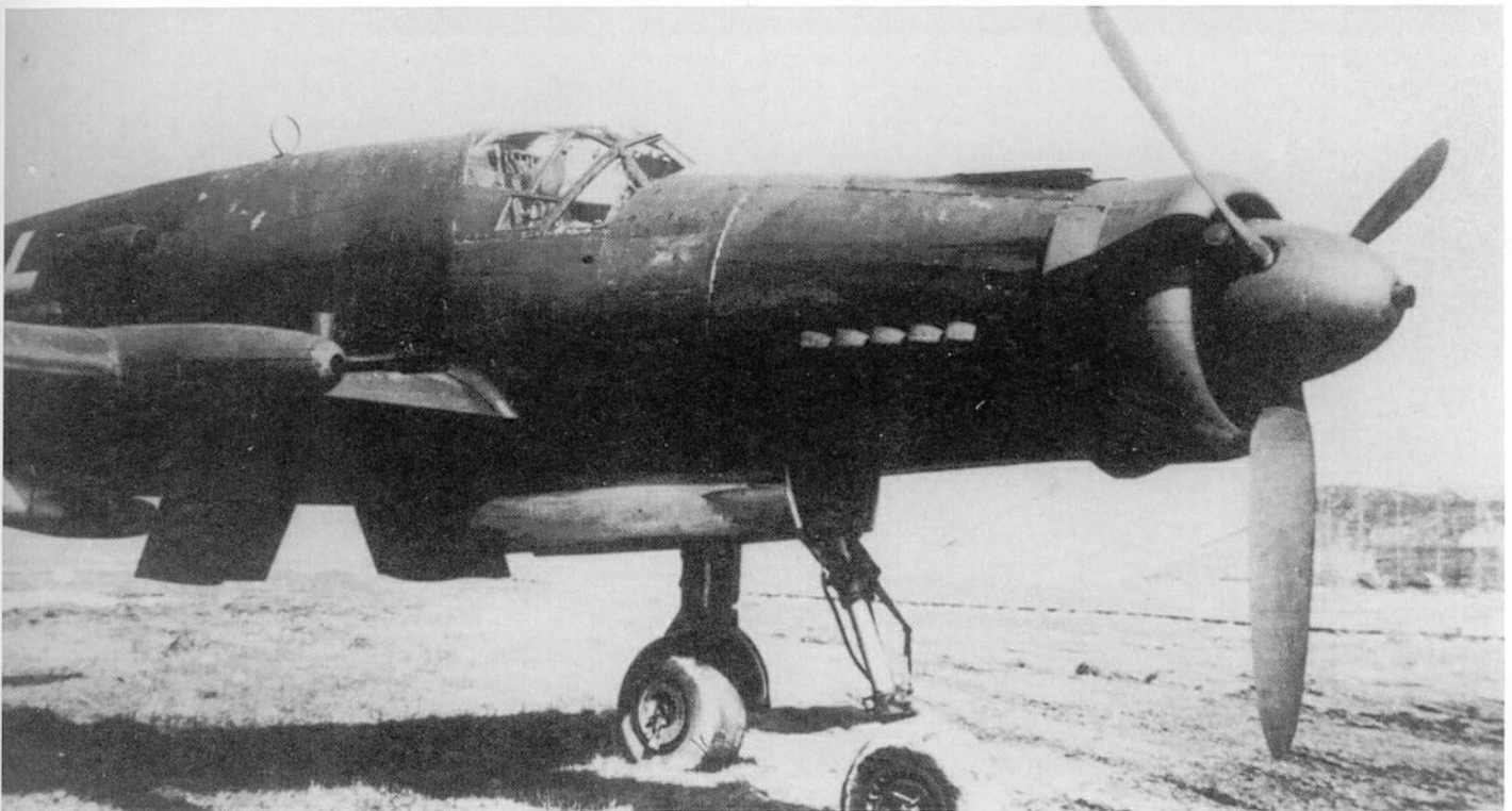
Below: The prototype Do 335 V-13 heavy-fighter ('RP+UA'), produced to the Building Requirement of 31 May 1944, with two additional MK 103s.
