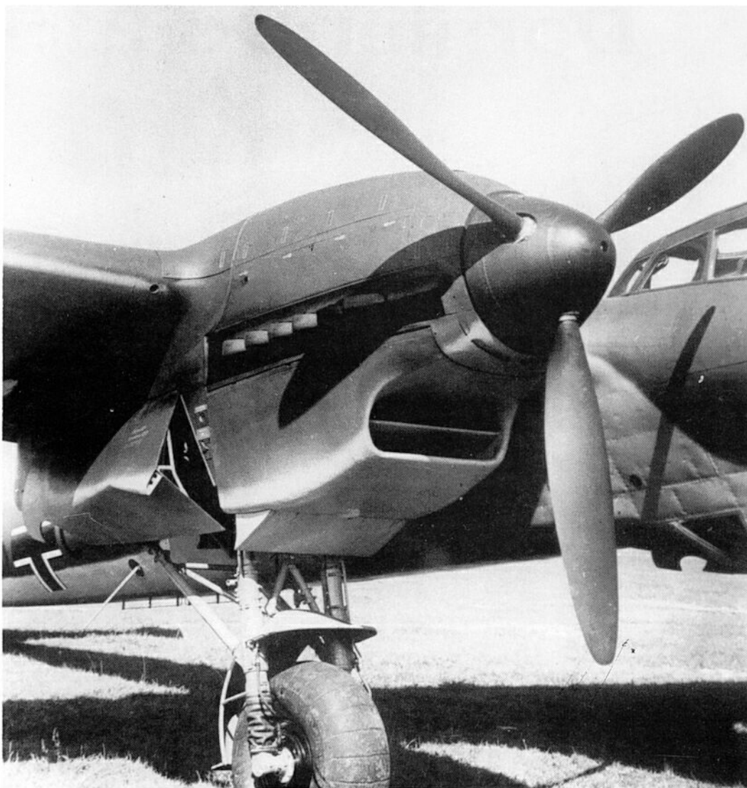
Left: The Do 215 B-1 was powered by two DB 601 Aa in-line engines. Most examples were used as long-range reconnaissance aircraft.
