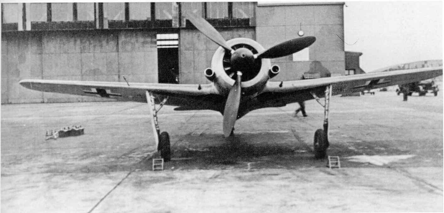
Below: The Fw 190 A-3/U7 went into production as a high-altitude fighter after only three test aircraft.
